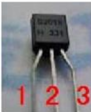
Pin arrangement of 9018, 8050
