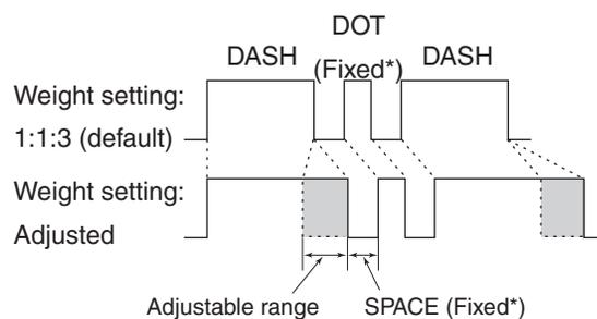
\*SPACE and DOT lengths can be adjusted with “KEY SPD” in the the Quick Set mode only.
