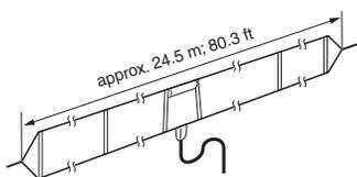
Covers from 1.9–30 MHz bands. Has an SO-239 connector. 30 m (98.4 ft) coaxial cable with PL-259 connector is supplied.
