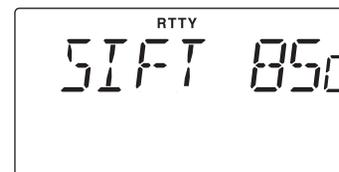
RTTY shift frequency is set to 850 Hz. 850, 425, 200 and 170 Hz can be used.
