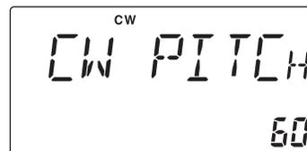
This shows the default setting for the CW pitch control (600 Hz).
