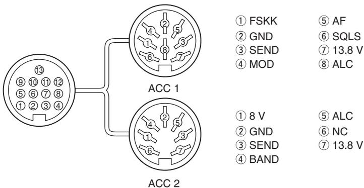
When the SEND terminal controls an inductive load (such as a relay), a counter-electromotive force can cause the transceiver to malfunction or other damage. To prevent this, we recommend adding a switching diode, such as an “1SS133,” on the load side of the circuit to the counter-electromotive force absorption. When the diode is added, a switching delay of the relay may occur. Be sure to check its switching action before operation.
