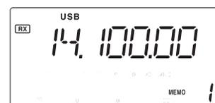
Memorized frequency (14.100 MHz) appears instead of the changed frequency (14.123 MHz).
