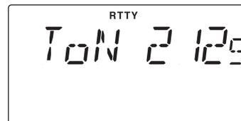
RTTY mark frequency is set to 2125 Hz. 2125, 1615 and 1275 Hz can be used.
