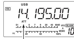
Appears when the attenuator is ON.
