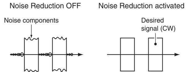
Higher setting of the [NR] level results in audio signal masking or distortion. Set the [NR] level for maximum clarity. The Noise Reduction function is usable in all modes.
