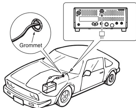
**NOTE:** Use terminals for the cable connections.
