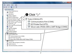
2 Check the COM port number. In this example, the USB serial COM port number is "3."
