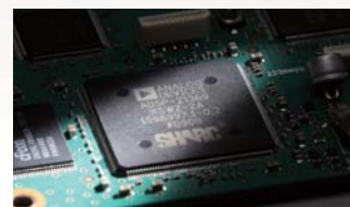
<DSP unit> ADSP-21369 Internal clock speed: 333MHz 32-bit floating point DSP Max. performance: 2000MFLOPS
